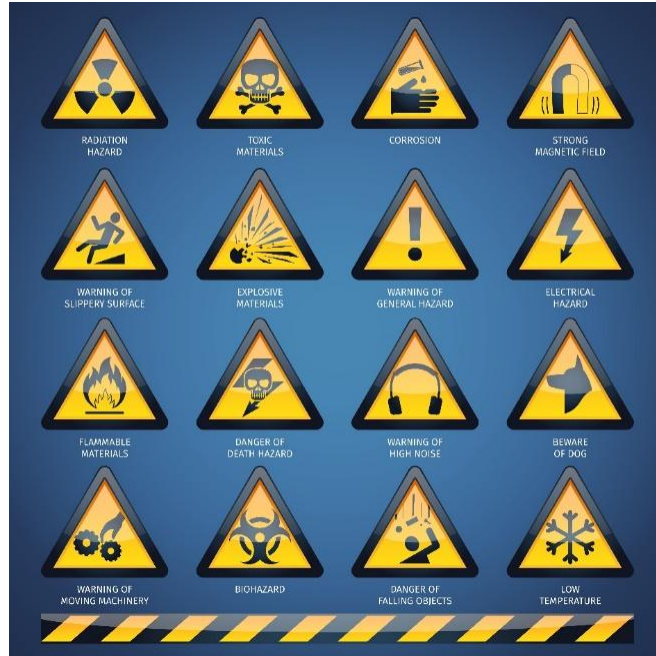
Fig. 4.12: Hazard Warning Signs
